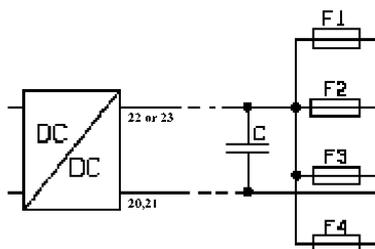
Figure 5. Connecting multiple loads.
