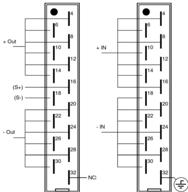
**Figure 1.** Pin-out on OUTPUT and INPUT DIN41612 H15 connectors.
