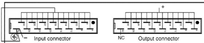
*Figure 9. Output to case isolation voltage test.*
